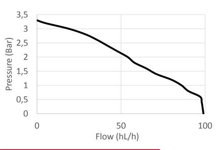
This test was carried out with a 3meter pipe Ø50, with water at 15°C. Pressure losses can be different, depending of the pipe and the characteristics of the product conveyed.
